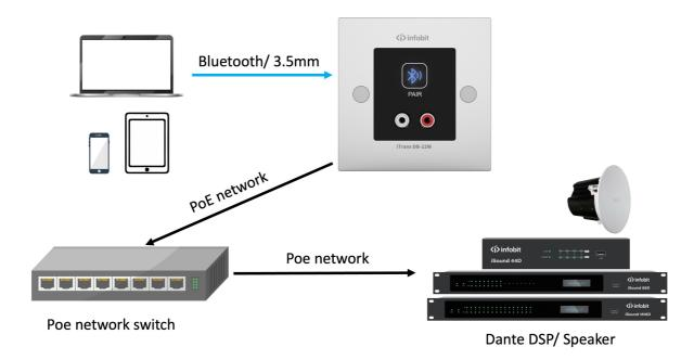
**Note:** The Bluetooth and RCA don't work simultaneously, the Bluetooth connection is priority.
