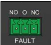
When the amplifier is working properly the NO / NC relay is activated in the normally closed position: NC.
