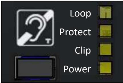
The unit is powered up using the gray switch on the front panel of the amplifier. If the amplifier is powered, the **Power** LED lights in blue.
